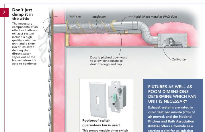
The installation of a ventilation system is critical. The duct system should take the shortest, most direct route to the outside; but even a short run of ductwork can be troublesome. To prevent trapped condensation, I use insulated, rigid pipe, and I make sure that the pipe has a slight pitch, either to the outside or back to the fan (detail 7 above).
